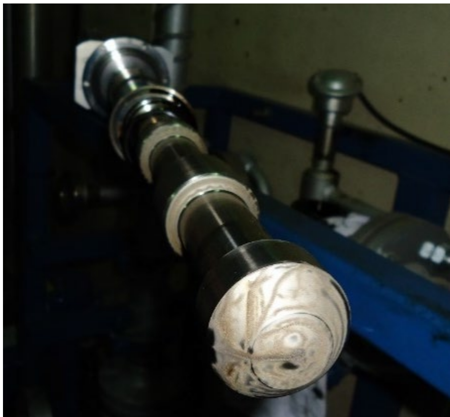
Figure 9 - Titanium sonotrode aspect after 6000 hours of operation. Cavitation marks on the working surfaces, evidencing material loss.
