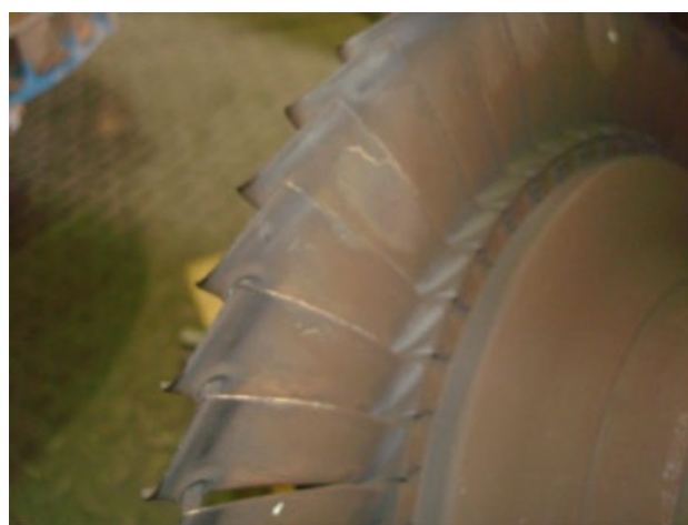
Turbocharger turbine 6,000h operation with HFO 380 cSt @ 50°C without fuel conditioning evidencing carbon deposits.
