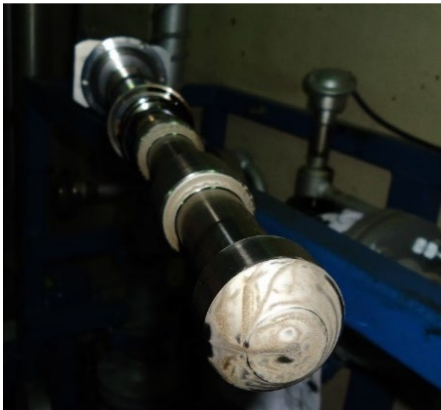
Figure 9 - Titanium sonotrode aspect after 6000 hours of operation. Cavitation marks on the working surfaces, evidencing material loss.
