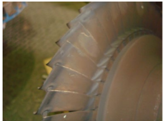
Turbocharger turbine 6,000h operation with HFO 380 cSt @ 50°C without fuel conditioning evidencing carbon deposits.
