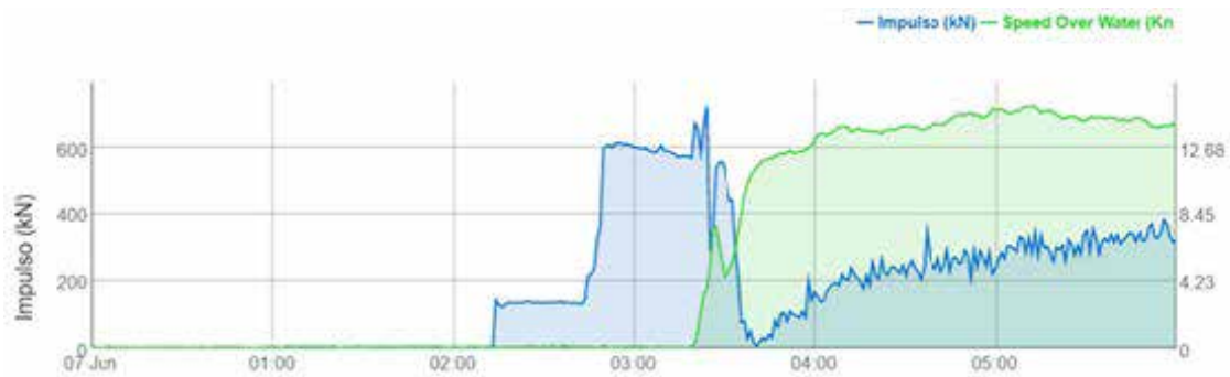
Img. 3 Graph showing Thrust and Speed Over ground as a function of time for a ship initiating a voyage in calm waters.
