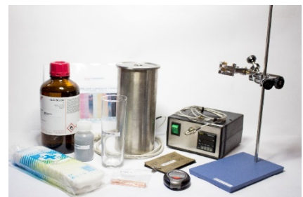
Figure 138 - Standard test method for corrosiveness to copper from petroleum products by copper strip test material.
