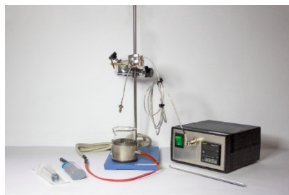
Figure 6 - Flash point and fire point determination in open cup test material.
