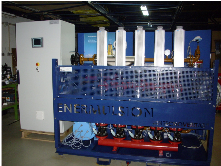
Figure 1 – General View of an Ultrasonic unit Enermulsion with a processing capacity of 4Ton/h.
