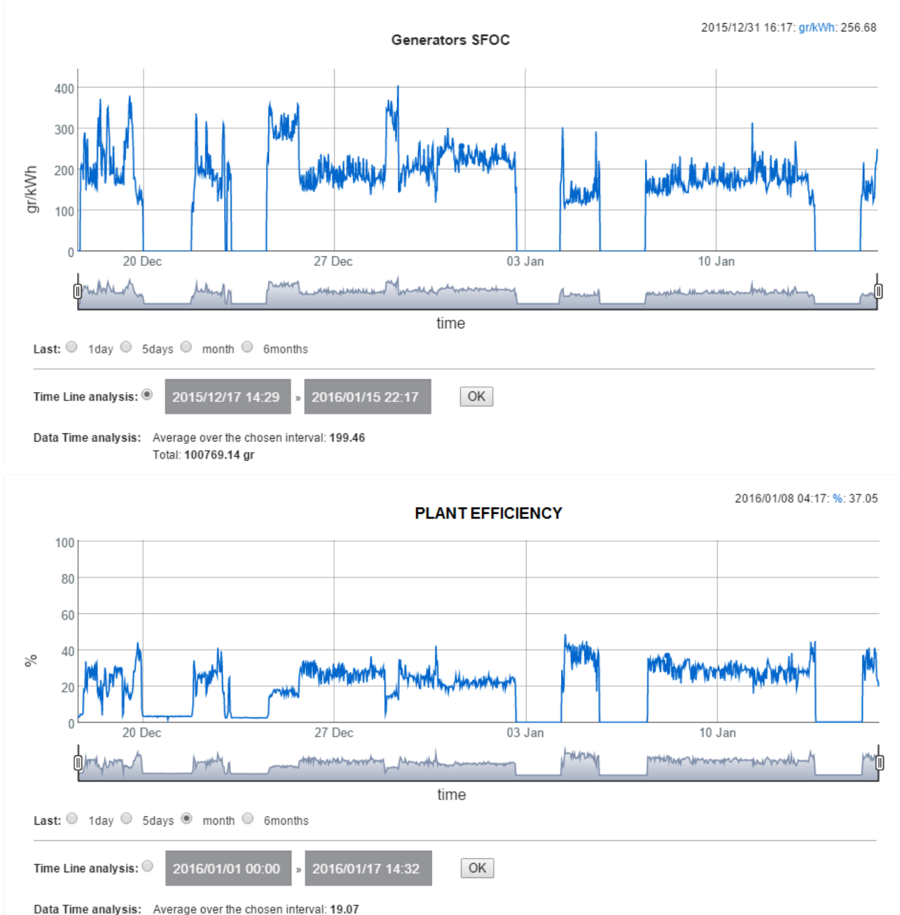
Img. 3 | Software BOEM-S: monitoring the specific consumption and performance of a Diesel installation along a function of time (1 month).
