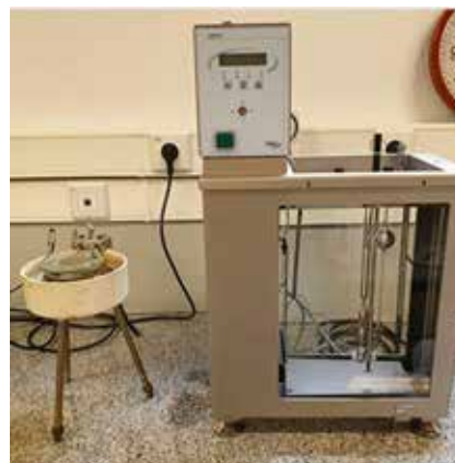
Figure 1 - Kinematic viscosity using Cannon Fenske calibrated viscometers or Ford cup calibrated viscometer.
