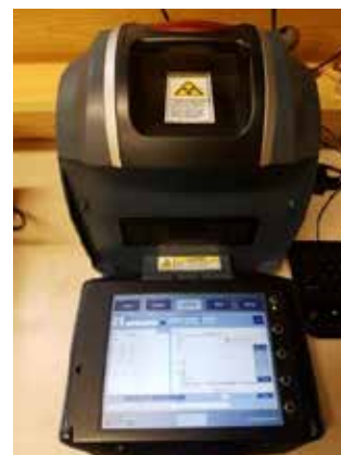
Figure 10 - X-Ray Fluorescence Spectrometer for determination of critical metals and elements
