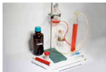
Figure 6 – Assembly for the Determination of water content by the petroleum column method.
