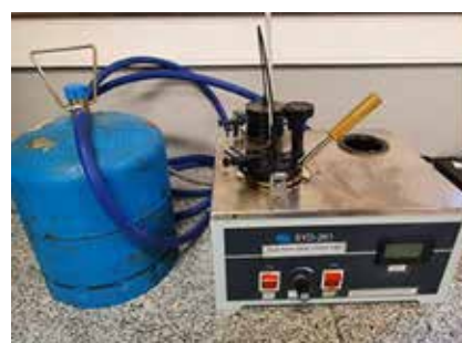
Figure 7 – Assembly for the Determination of the flash point by the Pensky-Martens closed cup method.
