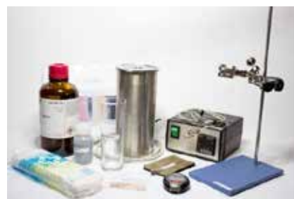
Figure 11 - Assembly for Standard Test Method for Corrosiveness to Copper from Petroleum Products by Copper Strip Test.
