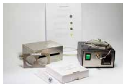
Figure 13 - Assembly for Insoluble content and degree of dispersion.
