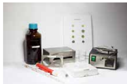
Figure 8 - Assembly for the Determination of Asphaltenes.
