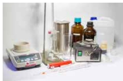
Figure 14 – Assembly for Standard Test Method for Acid and Base Number by Color-Indicator Titration.
