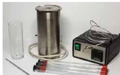
Figure 2 – Assembly for the Standard Test Method for Density, Relative Density, or API Gravity of Crude Petroleum and Liquid Petroleum Products by Hydrometer Method.
