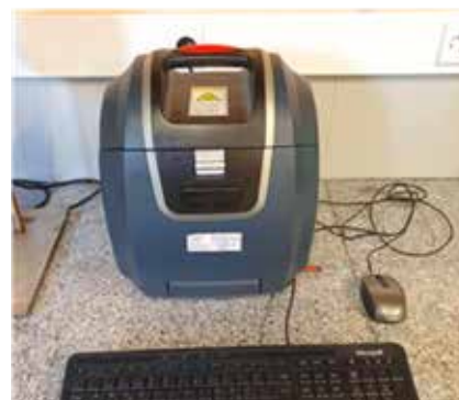
Figure 9 – Assembly for the Energy-dispersive x-ray fluorescence spectrometry: sulphur determination, critical metals, and elements monitoring.
